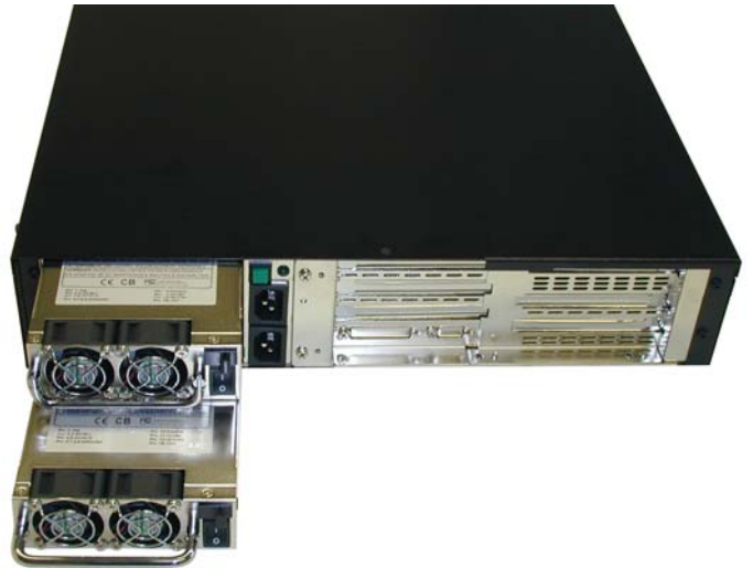
RM-298C installed Redundant Power
