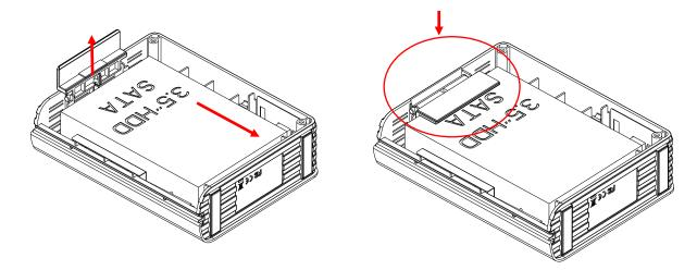
5. Close the aluminum plate and fix the screws back to the case
