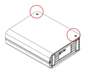
2. Detach the aluminum plate and see internal structure
