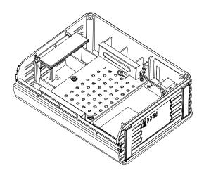
3. Open the HDD flip locker
