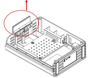
4. Slide the HDD to attached the connector and close the flip to fix the HDD
