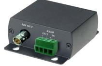
SR02 is a repeater for HD-SDI links operating with  $75\Omega$  coax cable. It can be daisy chained together up to 5 pieces of SR02 with working distance 1KM. When using multiple SR02 repeaters installation, the repeater power could be send over coax cable from the remote repeater (nearest the DVR). It also support RS485 data control as well. The application could be using for HD CCTV HD-SDI camera extra long range video monitoring.
