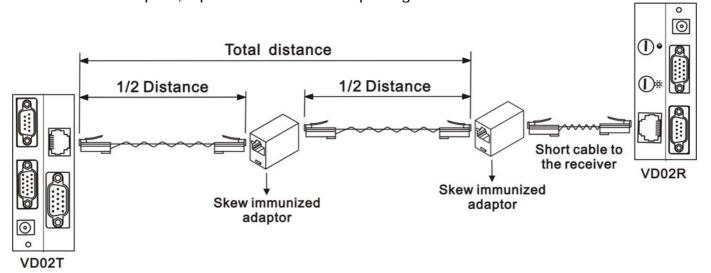
CAUTION: to avoid display equipment damaged, be sure to make correct cable connection and power for both VD02T before connecting VD02R
