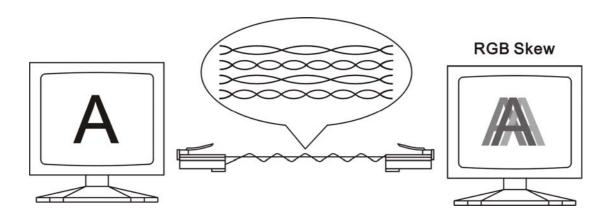
1. Recommend to use following cabling way to reduce skew status, to add special made "skew immunized adaptor", 2 pieces included at the package.
