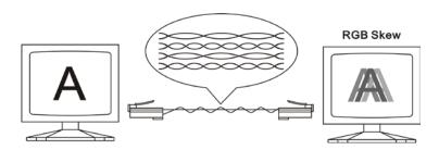
2. Recommend to use following cabling way to reduce skew status, to add special made "skew immunized adaptor", 2 pieces included at the package.
