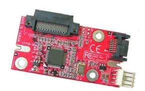
Slim Optical Device --- > Serial ATA Optical Drive!
