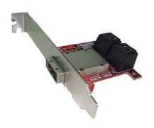
Ideal Low Profile PCI Adapter that converts onboard Internal 4Ports SAS or SATA to mini-SAS SFF-8088 connector for external connection!
