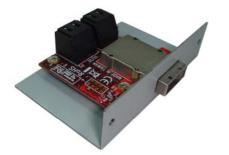
External connection the single mini-SAS SFF-8088 port in SCSI-1 form factor to 4 units of 7Pin SAS or SATA Drive!
