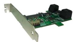
5Ports 6Gbps SATA Port Multiplier Low Profile Host Adapter expands main board Port Multiplier compatible SATA one port to connect 5 units of SATA Device!
