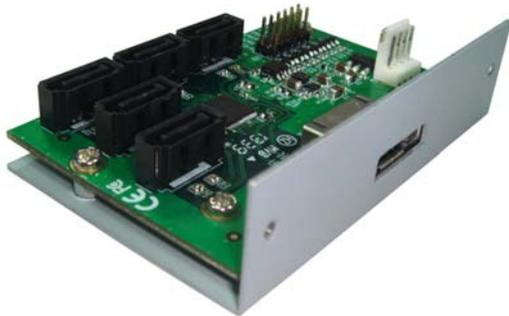
**6Gbps SATA III based SCSI-1 Centronic 50Pin form factor Adapter for 5Bay Rack Mount Storage System that Connects 5 units of SATA I & II & II device to one port
