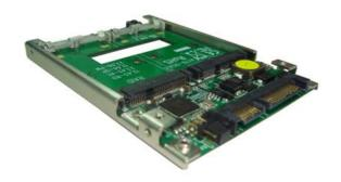
Best Solution that Easily Latch and Retain Fast Speed 2x mSATA SSD to normally standard 7mm 2.5 inch SATA III Solid State Drive with H/W RAID functionally!
