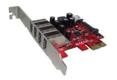
External 4 Port USB 3.0 SuperSpeed 5Gbps in Low Profile PCIe Host Adapter to support all kind of 5Gbps, 480Mbps, 12Mbps and 1.5Mbps USB Devices!
