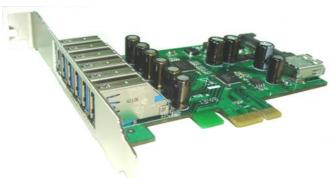
External 6 Ports and Internal 1 Port USB 3.0 SuperSpeed 5Gbps in Low Profile PCle Host Adapter to support all kind of USB 3.0, USB 2.0, USB 1.1 Devices!
