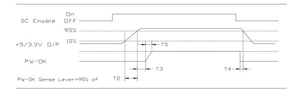
Timing of PS-ON, PW-OK, and Germane Voltage Rails
